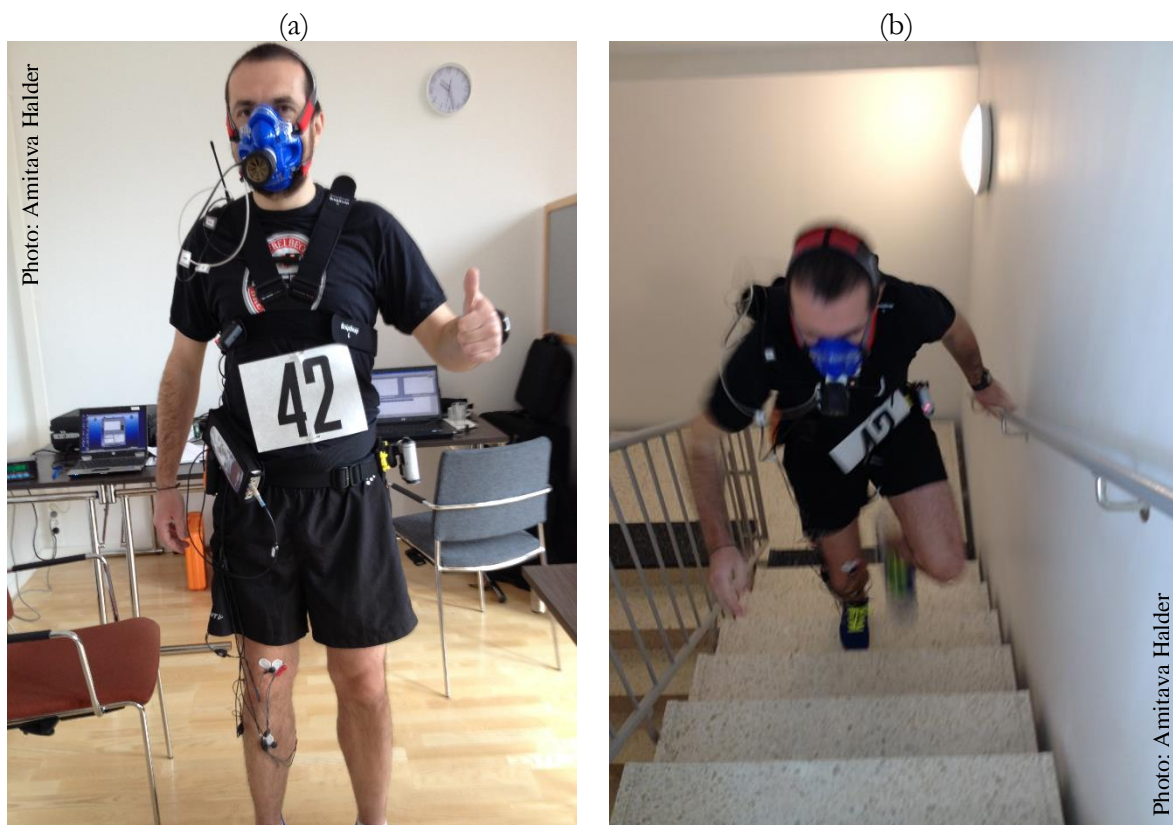
Figure 5. A fully equipped test participant before (a) and during the ascending evacuation test (b).
