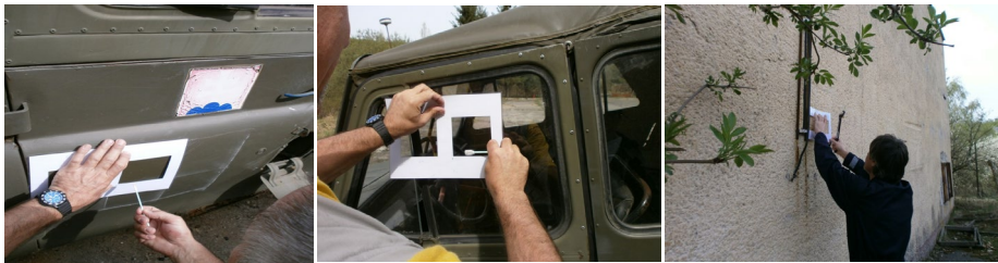
Figures 8-10. Collecting samples from vehicle door, window and wall
