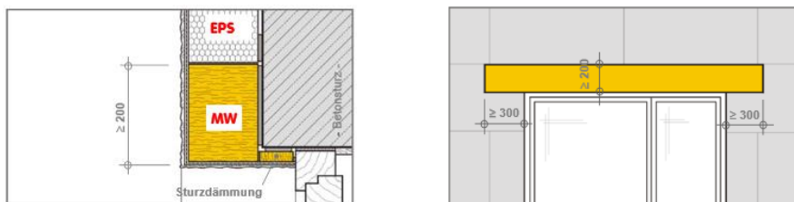
Figure 11 – Barrier at the lintel of opening – specimen S2
