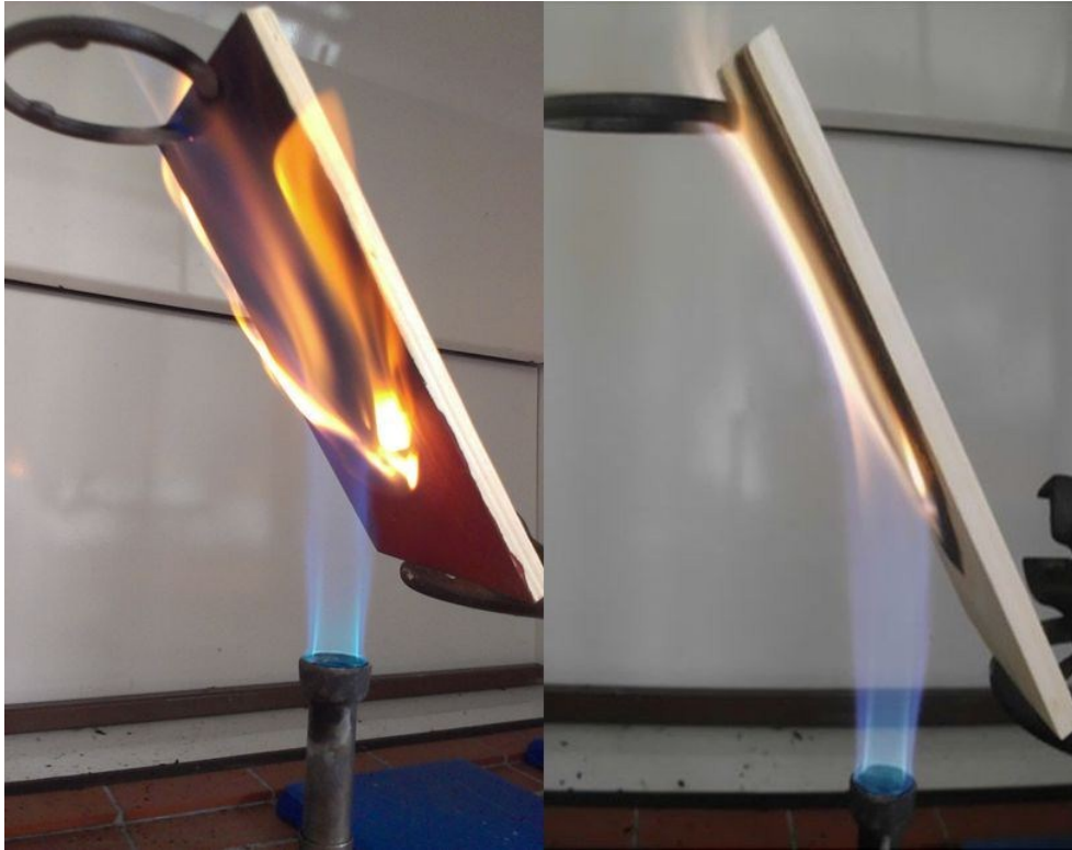
Figure 3. The realization of experiment - test specimens during the test of limited flame spread.
