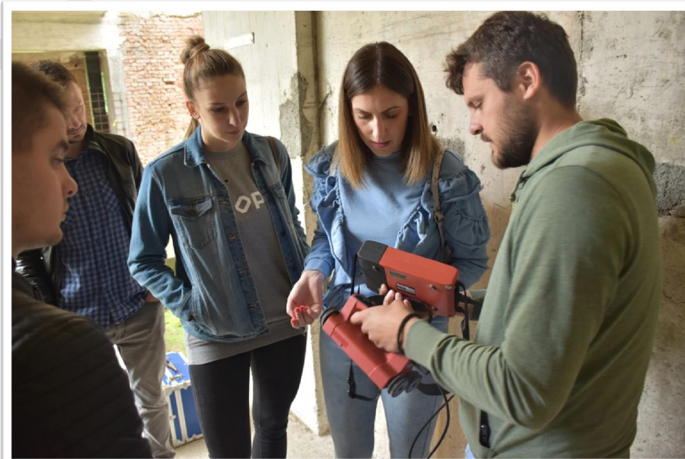
Multi Functional Rebar Detector testing in existing concrete structure
