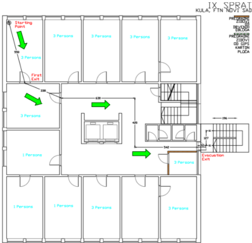
Fig 4.1 Evacuation route for the 9 th floor
