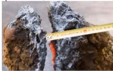
Figure 1 – Molten decomposed concrete [7]
