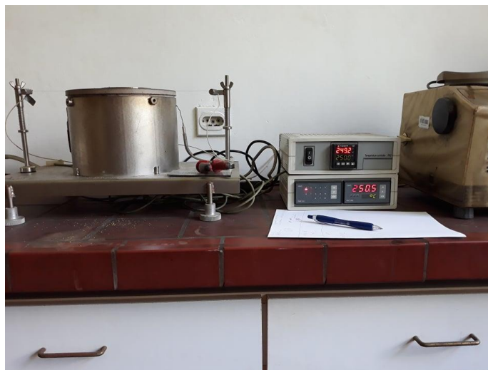
Figure 3.-Self-ignition temperature measuring apparatus
