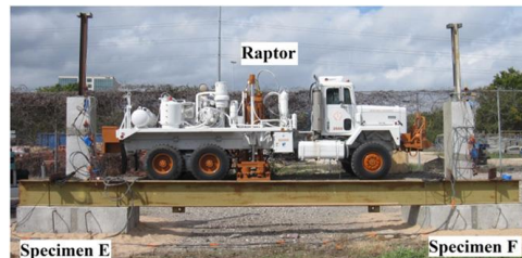
Figure 20 – Experimental setup for 1D metamaterial foundation
