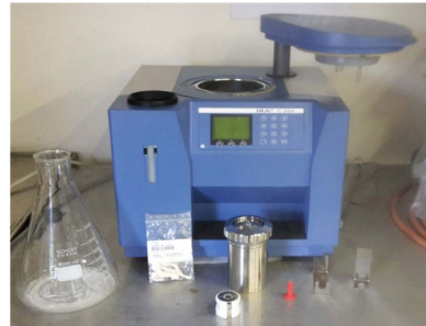
Figure 5 – bomb calorimeter parts
