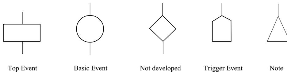
**Figure 4.17: Symbols commonly used in fault tree representations.**
