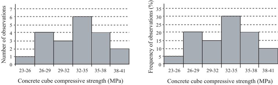
**Figure 2.4:** Histogram and frequency distribution representations of the observed concrete cube compressive strength.
