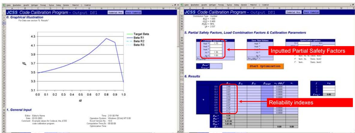
Figure 8. Graphical illustration and table of computed reliability indexes.
