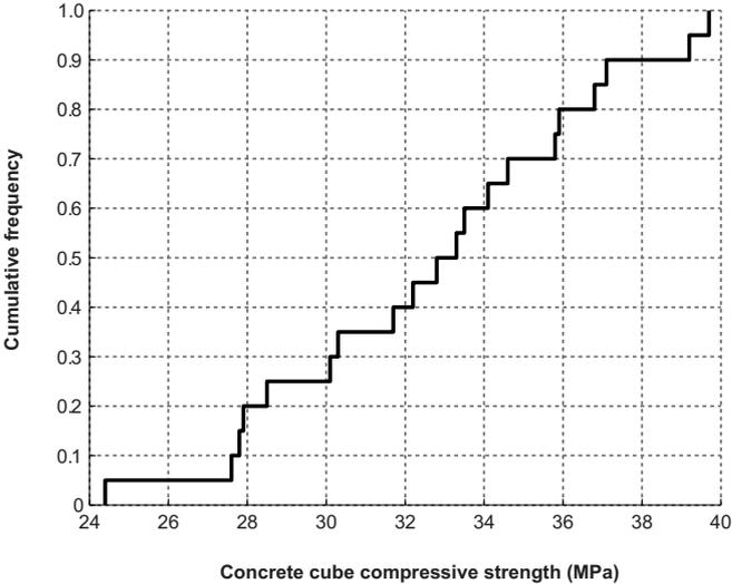
**Figure 2.5:** Cumulative frequency plot of the observed concrete cube compressive strength.
