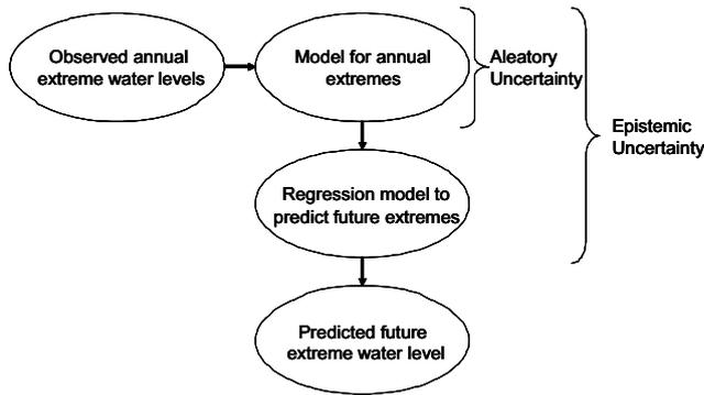
**Figure 2.9: Illustration of uncertainty composition in a typical engineering problem.**
