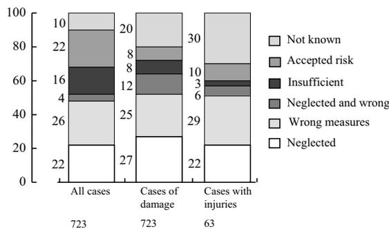
**Figure 1.12: Illustration of the relative distribution of causes of failures and errors (Matousek and Schneider (1976)).**
