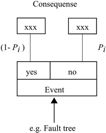
Figure 4.24: Gate in a cause consequence chart.
