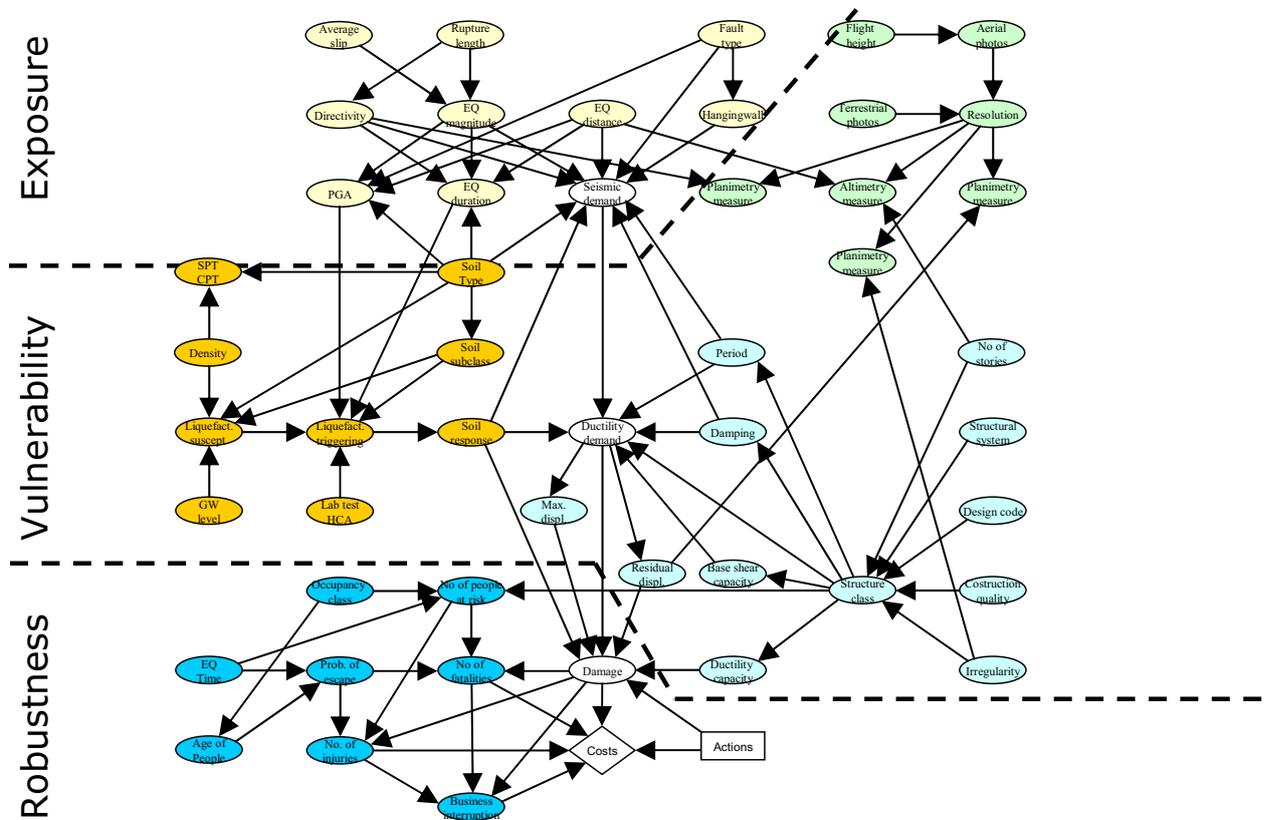
Figure 10.17: Generic indicator based BPN for the assessment of earthquake risks for one building class.
