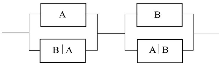
**Figure 9.9: Block diagram for the systems reliability analysis of the beam structure at level 2 (or mechanism level).**
