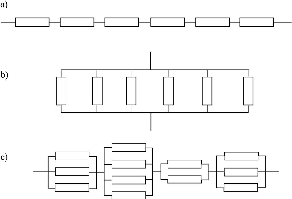
**Figure 9.2:** Block diagrams used in the reliability analysis of structural systems.
