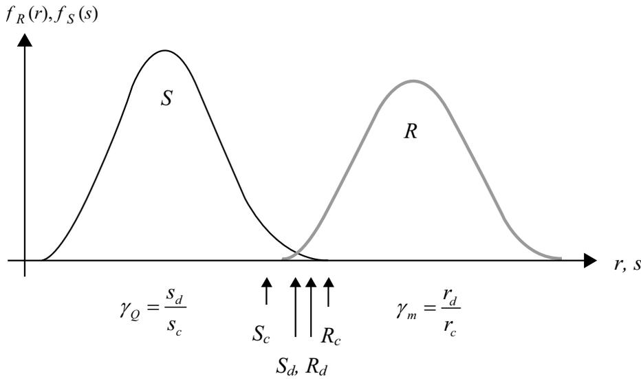
**Figure 6.3: Illustration of the relation between design values, characteristic values and partial safety factors.**
