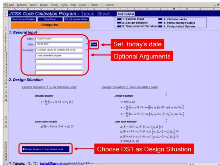
Figure 4. Definition of general input and design situation.
