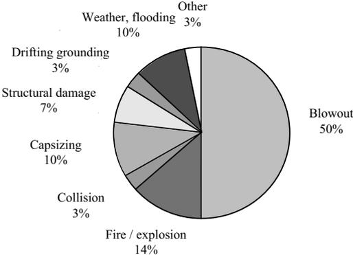
**Figure 1.22: Distribution of initiating events for failures of submersible rigs (Bertrand and Escoffier (1987)).**
