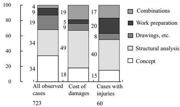
**Figure 1.15: Illustration of the distribution of the phases during planning where risks were inadequately treated (Matousek and Schneider (1976)).**
