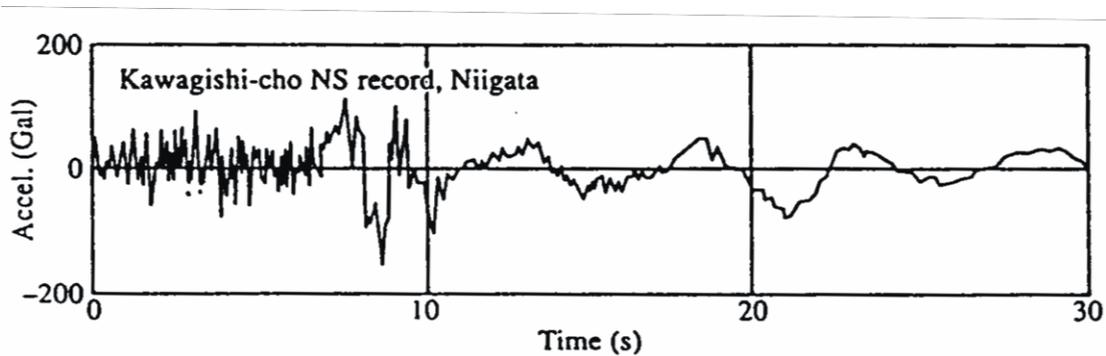
Fig.3.10 Niigata earthquake motion on liquefied ground; probably affected by soil softening after 8 seconds
