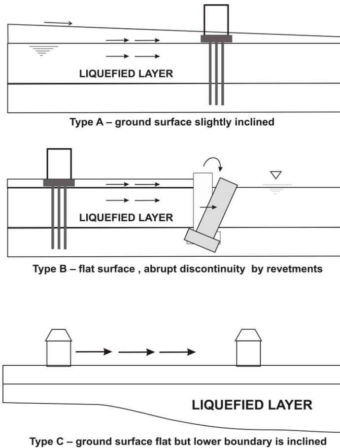
Fig. 3.4. Types of lateral ground displacements, after Hamada et al. 1986
