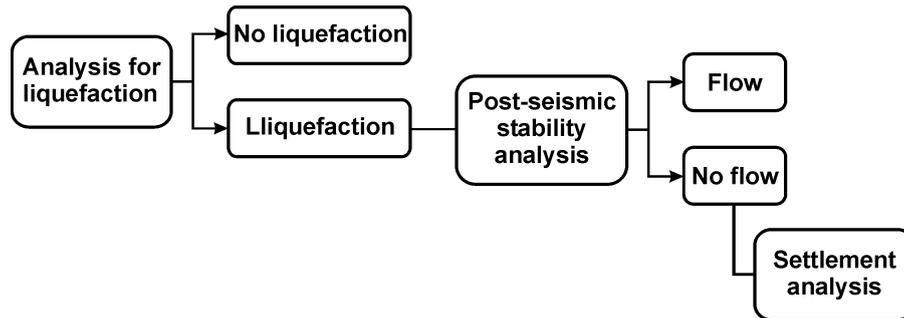
Fig.3.2 Flow chart of the problems associated with liquefaction (Ishihara, 1993)
