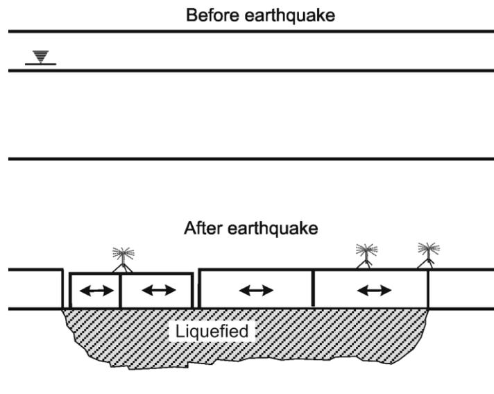
Fig.3.5. Diagram of horizontal ground oscillation cause by liquefaction in the cross-hatched zone decoupling the surface layer from underlying ground
