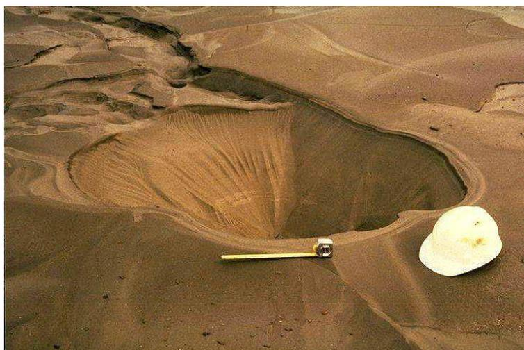
Fig. 3.9 Sand boil, during the Loma Prieta Earthquake , USA (1989, M = 7.1)
