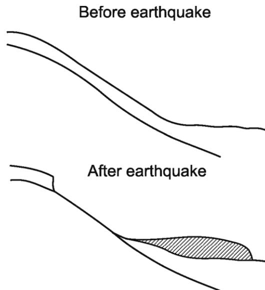
Figure 3.3 Diagram of flow failure caused by liquefaction and loss of strength of soils lying on steep slope. The strength loss creates instability and flow down the steep slope
