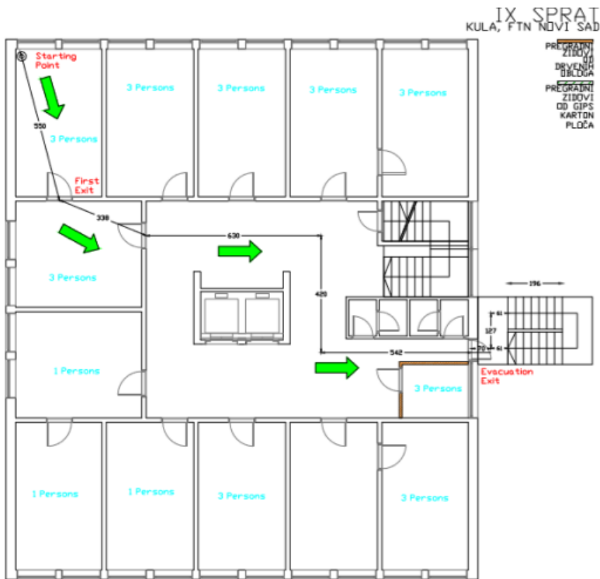
Fig 4.1 Evacuation route for the 9 th floor
