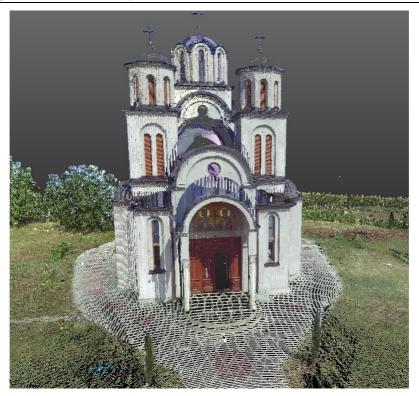
Figure 7 – Point cloud generated using TLS technology
