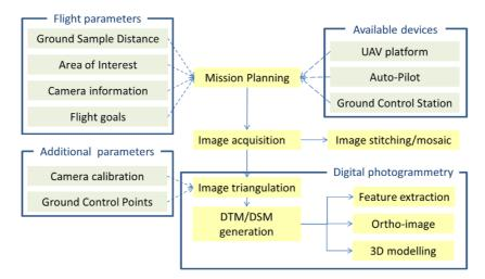
Figure 3 – General workflow for acquisition and processing of UAV images [7]
