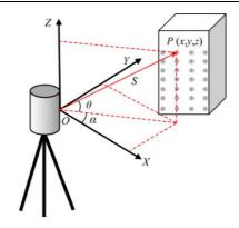
Figure 8 – Measuring principle of the terrestrial laser scanning [14]
