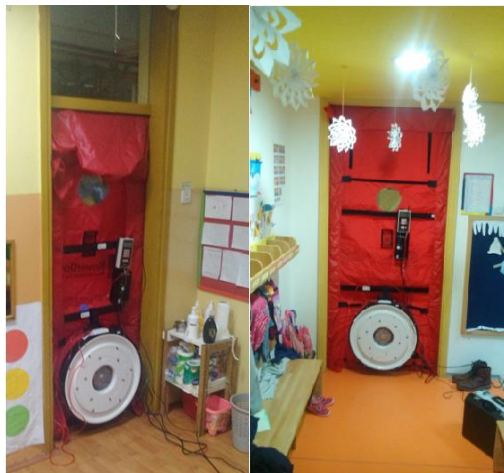
Figure 6 – Blower door test measurement
