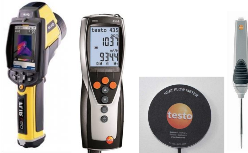
Figure 4 – FLIR b60 (left) and TESTO 435-2 for U-value measurement with fluxmeter and temperature sensor (last 3 images on the right)
