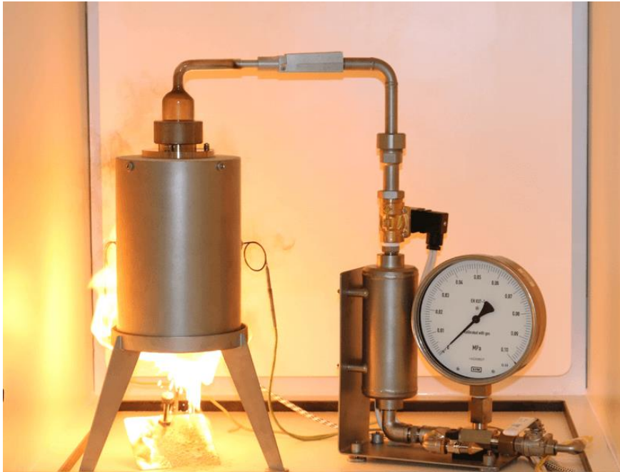
Figure 8 – Scheme of equipment for measuring ignition temperature of whirled dust ( https://www.sigma-hse.com/process-safety-testing/dust-and-powder/minimum-ignition-temperature-mit )
