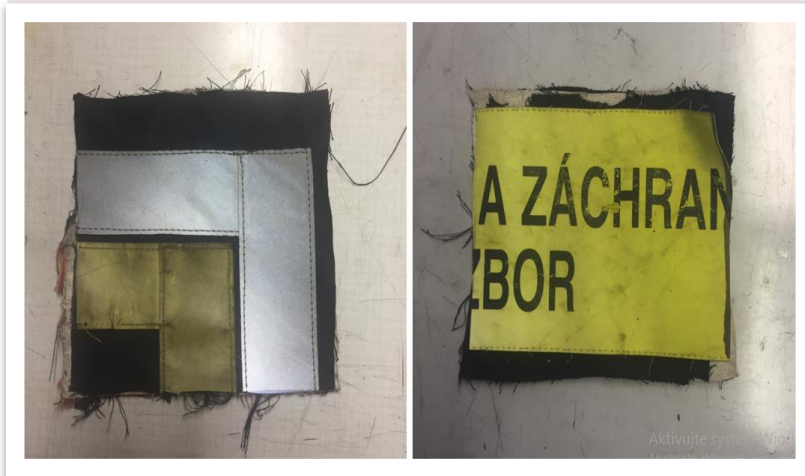
Test specimen with reflective strips and inscription
