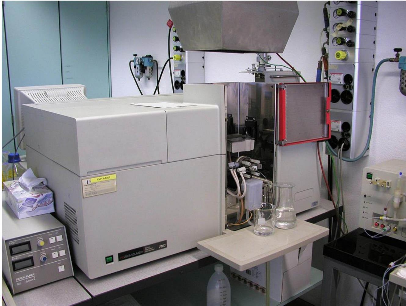
Flame atomic absorption spectroscopy instrument, https://commons.wikimedia.org/wiki/File:FlammenAAS.jpg#/media/File:FlammenAAS.jpg , 02.05.2019.
