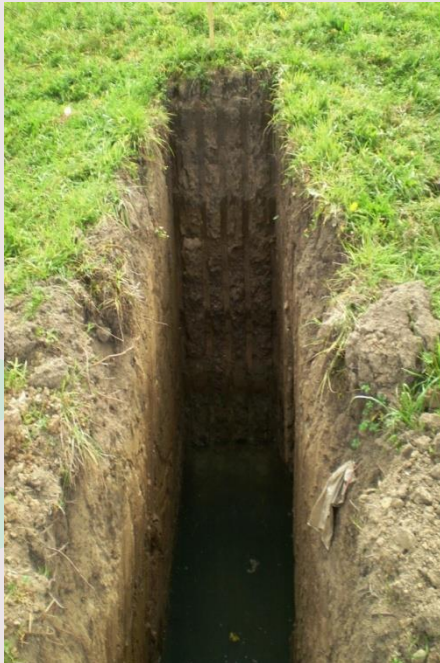
Probe ditch for sampling
