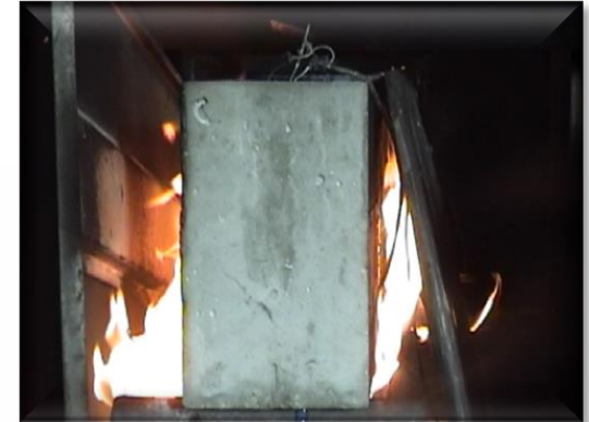
Fire testing of beam specimen
