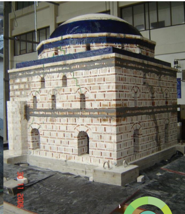
strengthened by CFRP bars & wrap
