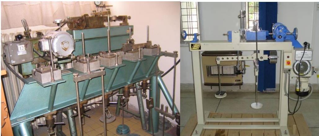
Figure 14. Shear device with defined shear plane (controlled force increment and controlled deformation increment.)
