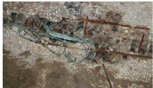
Fig. 17. Local deep overheating of concrete and deformed rebars due to wirings within cross-section (a – beam, b – slab)
